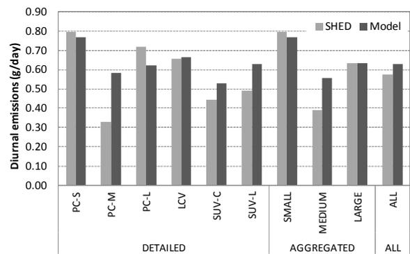
Figure 2. Modelled vs tested diurnal emissions for ADR79-01 and ADR79-00 vehicles combined.
