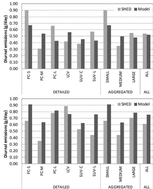
Figure 1. Modelled vs tested diurnal emissions for ADR79-01 (top) and ADR79-00 (bottom) vehicles.
