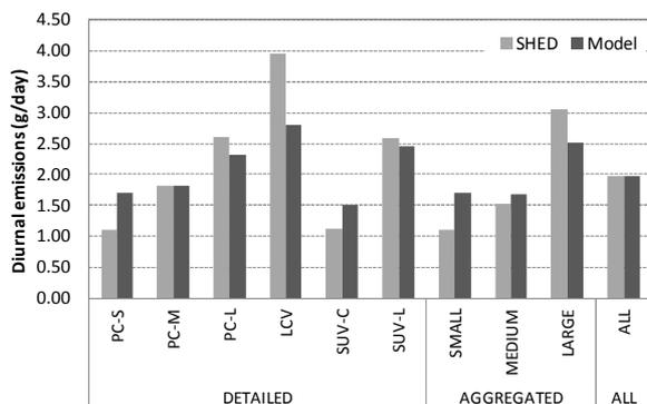
Figure 3. Modelled vs tested diurnal emissions for ADR37-01 vehicles.
