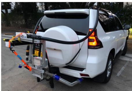
Figure 2. PEMS testing in Sydney.
