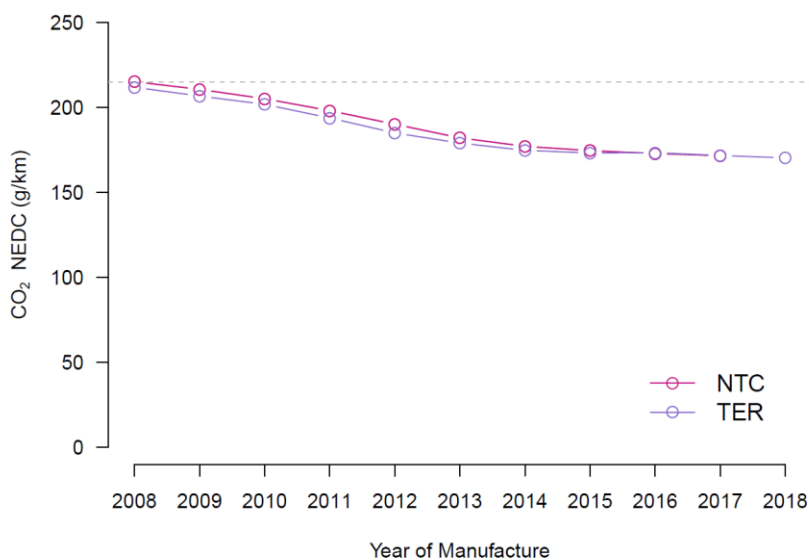
Figure 3 – Reported ‘official’ average CO 2 emission rates for the new PV fleet, TER vs. NTC (NEDC).
