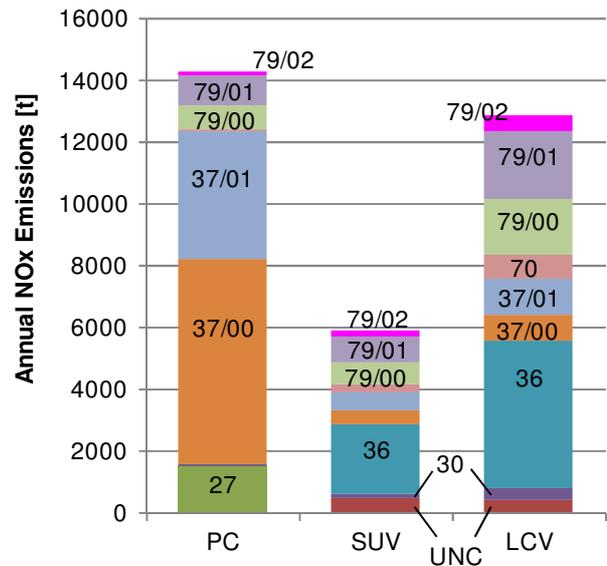
Figure 1. Contribution of different emission control technologies to total NO<sub>x</sub> emissions for selected vehicle categories.
