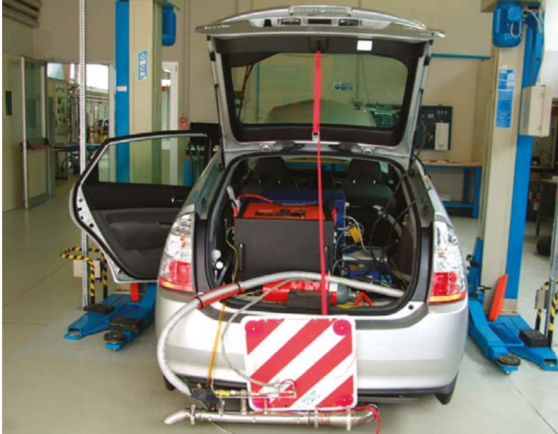
Figure 10.2 PEMS emission-testing set-up for LDVs (reprinted from Weiss et al., 2011, p. 8575)
