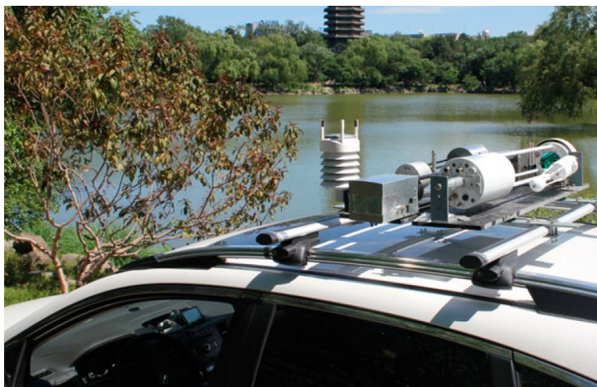
Figure 10.12 Open-path sensors on vehicle roof (reprinted from Sun et al., 2014, p. 3943)
