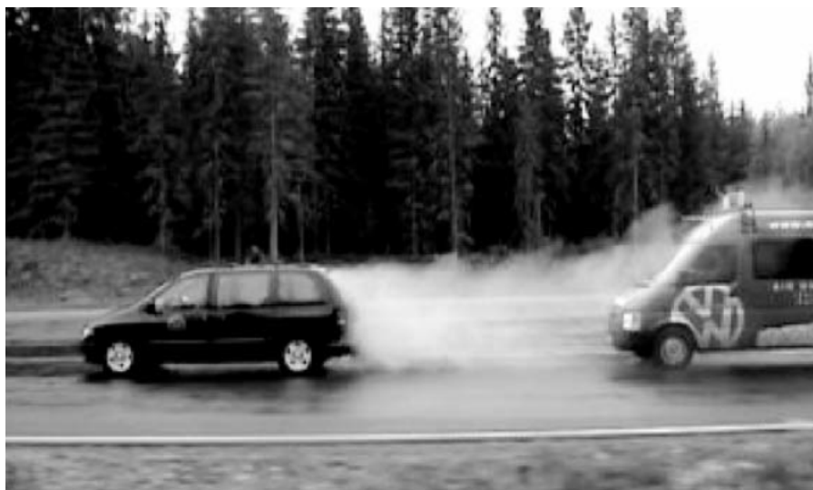
Figure 10.10 Exhaust plume measurement test (reprinted from Pirjola et al., 2004, p. 3628)
