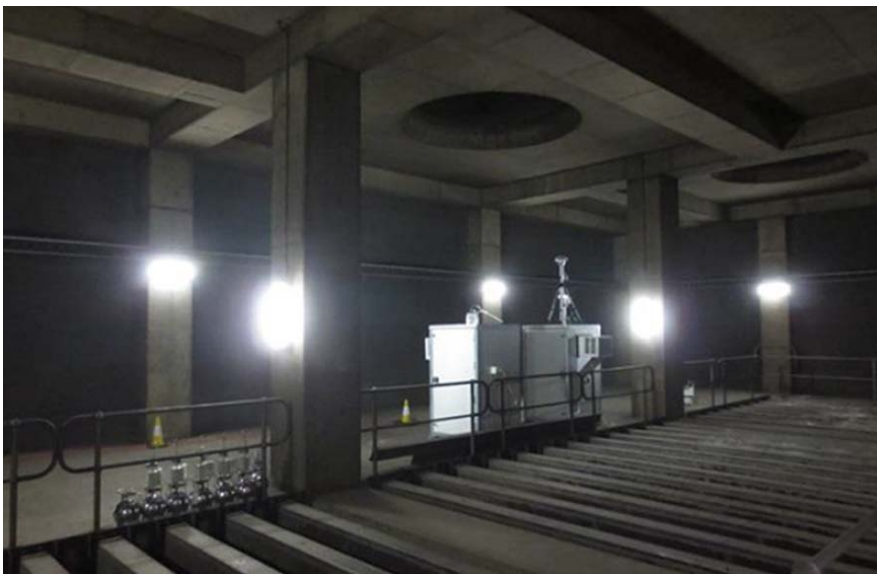
Figure 10.4 Concentration measurements within tunnel ventilation system (reprinted from Smit et al., 2017, p. 190)
