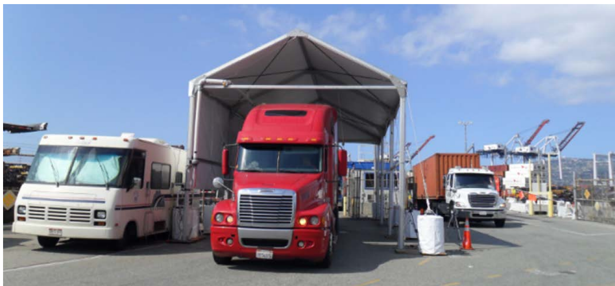
Figure 10.9 On-road system for HDV emissions monitoring (reprinted from Bishop et al., 2015, p. 1639)
