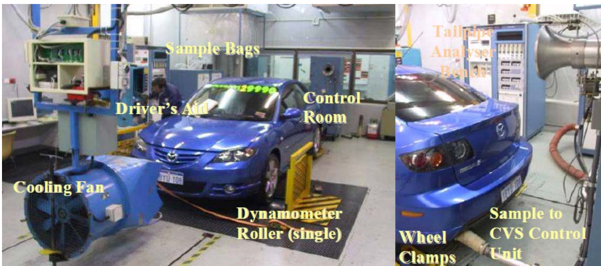
Figure 10.1 Laboratory emission-testing set-up (reprinted from Orbital, 2009, p. 37)
