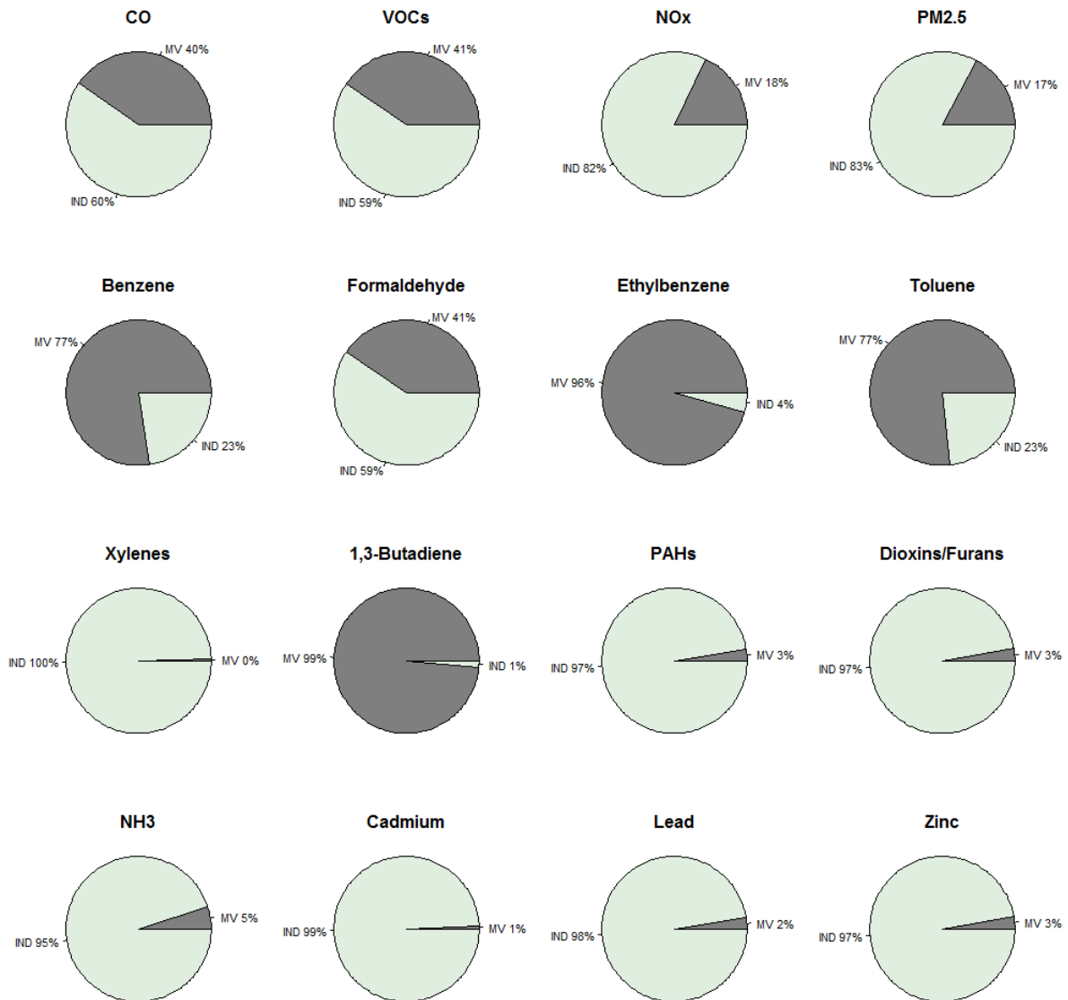
Figure 11 Contribution of motor vehicle (MV) and industry (IND) emissions to their combined total emissions
