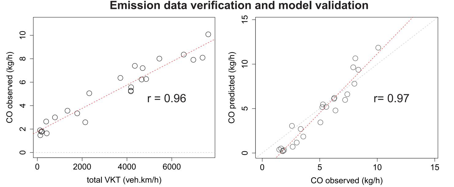
Vehicle emission prediction software is well-developed in Europe and the US. However, they do not adequately reflect Australian conditions (fleet mix, vehicle technology, fuel quality, climate) therefore two software packages were recently developed (2013) using data from major Australian emission testing programs (~ 2500 modal vehicle emission tests and ~ 12,000 vehicle emission bag tests).
