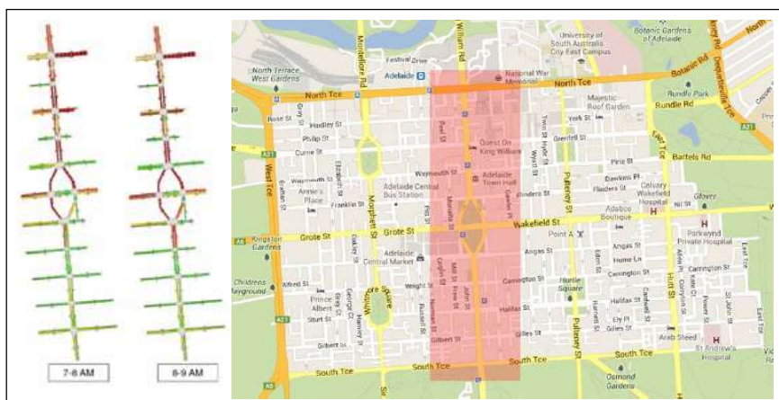
Figure 4: Predicted total NO x emissions for different road segments in part of the Adelaide CBD network for two morning peak hours (Smit, 2013)
