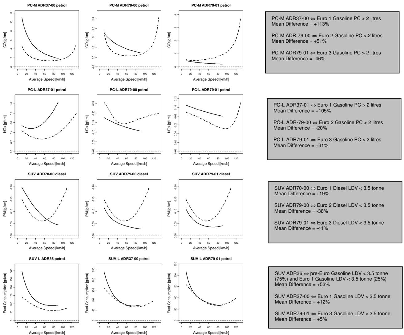
Figure 5: Comparison between COPERT Australia 1 (Solid Line) and COPERT 4 (Dashed Line) Hot Running Emission Factors for a Selection of LD Vehicle Classes and Pollutants, Grey Boxes on the Right Contain Information on the Corresponding Vehicles Classes in Both Models and the Average Difference (Range 10-90 km/h).
