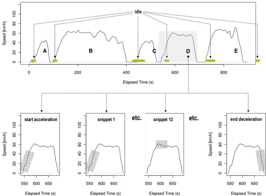
Figure 3: Schematic of Segmented Database Creation.
