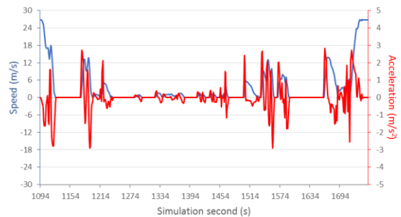
Fig. 1. Speed-acceleration-time profile for a car in a saturated traffic scenario -S1- in Brisbane (Australia)
