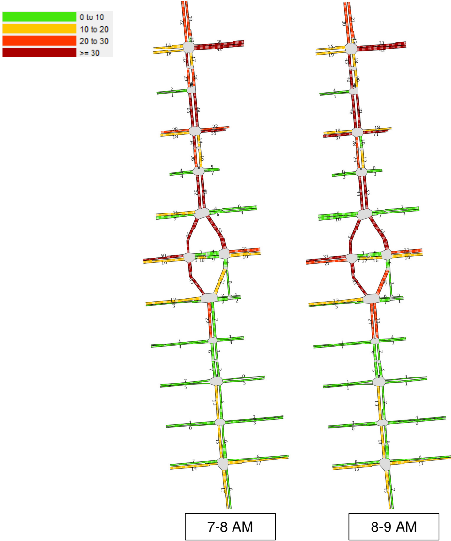
Figure 3: Predicted Total NO x Link Emissions in the Network for Two Time Periods (07:00-08:00, left chart, and 08:00-09:00, right chart)
