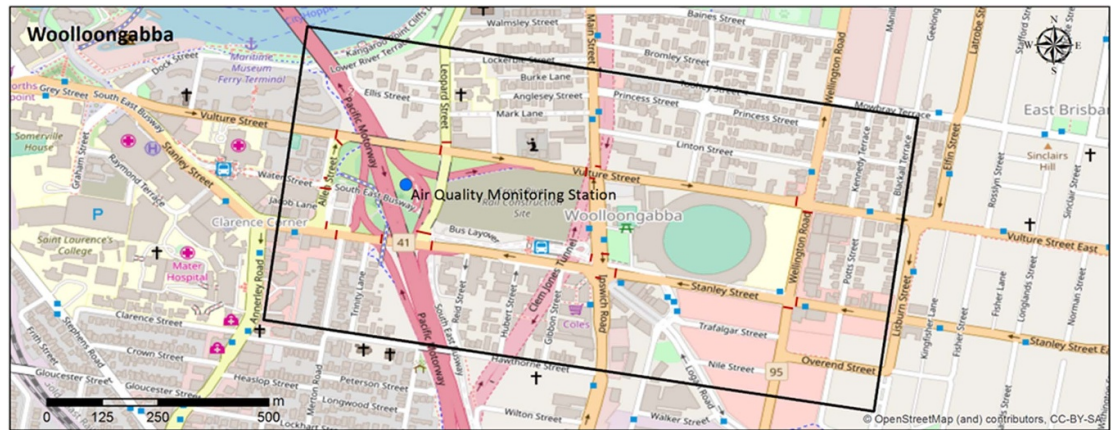
Figure 2. Traffic microsimulation domain of 1250 m × 600 m (black rectangle) for Woolloongabba area with red lines for traffic lights. Reproduced with permission from (Quaassdorff 2018). CC BY-NC-ND 4.0.
